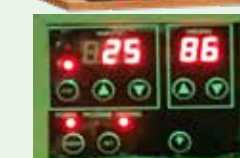
Fig1. POWER & HEATING lights illuminated to show sauna in operation
